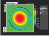
RWE of 5" narrow band pass filter at 780nm
