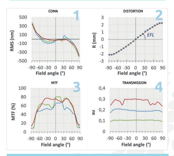
Aberrations of a complex zoom lens with high NA (F/2) 450 nm 530 nm 660 nm
