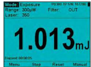
Exposure measurement (energy summing) with photodiode sensor.
