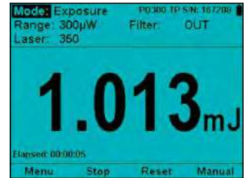
Exposure measurement (energy summing) with photodiode sensor.
