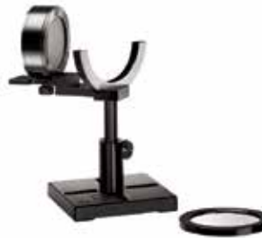
Beam Splitter removed – direct beam on sensor
