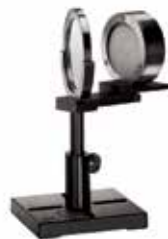
Beam splitter installed – reflected beam on sensor
