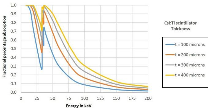
X-ray absorption efficiency for indirect detection version
