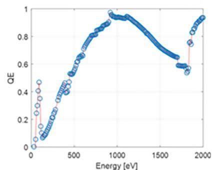
Quantum Efficiency for direct detection version
