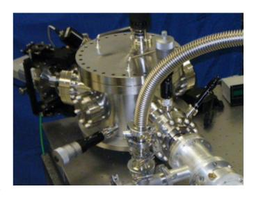
ray (SXR, XUV), extreme ultraviolet (EUV), and VUV. This is a practical instrument for applications requiring rapid data collection from transient, short lived events. Examples include fusion plasmas (http://www.pppl.gov/LTX) formed in tokamak devices, laser ablation, liquid droplet EUVL sources (http://www.xuv.com/xenon.html), and Xenon plasma at 13.5nm (http://www.cymer.com/plasma-chamber-detail) considered for extreme ultraviolet lithography.
